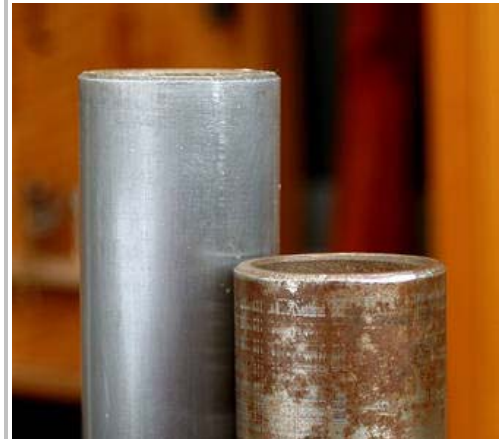
The steel tube in the background was once as rusty as the one in the foreground. We removed the rust with a chemical chelator.
