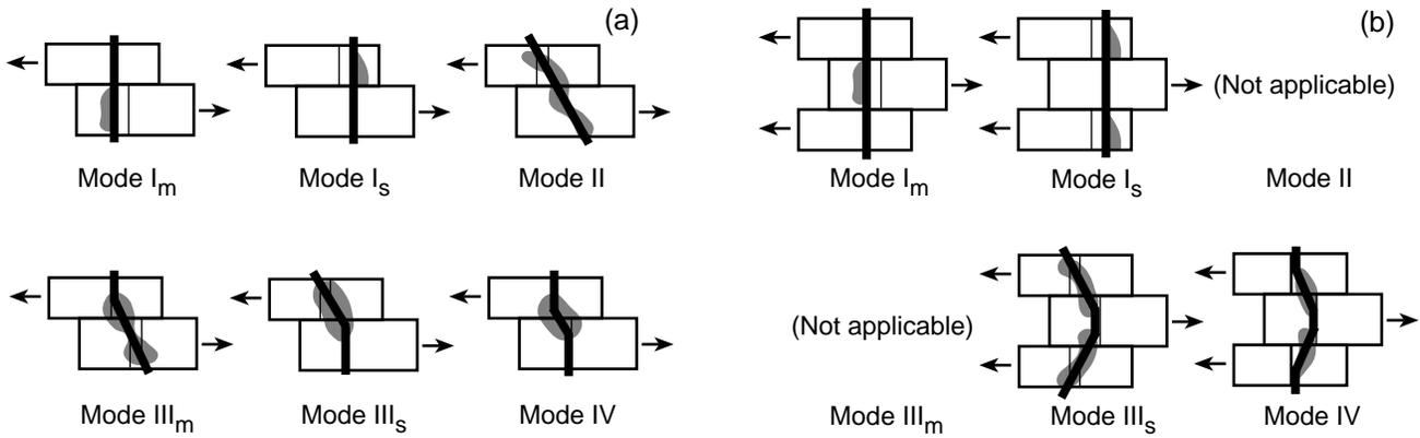
**Figure 7-4. Various combinations of wood-bearing and fastener-bending yields for (a) two-member connections and (b) three-member connections.**
