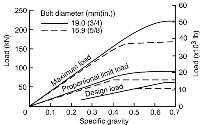
**Figure 7-20. Relation between load bearing parallel to grain and specific gravity (ovendry weight, volume at test) for two 101.6-mm (4-in.) shear plates in air-dry material with steel side plates. Center member thickness was 88.9 mm (3-1/2 in.).**
