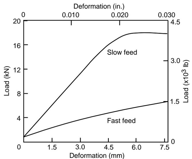
**Figure 7–14. Typical load–deformation curves showing the effect of surface condition of bolt holes, resulting from a slow feed rate and a fast feed rate, on the deformation in a joint when subjected to loading under bolts. The surface conditions of the bolt holes were similar to those illustrated in Figure 7–13.**
