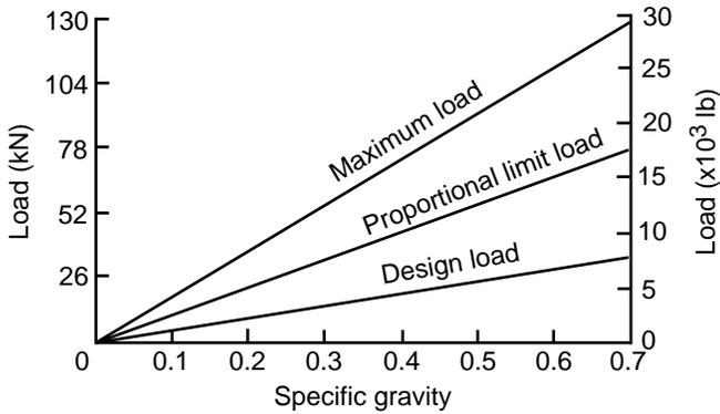
**Figure 7-17. Relation between load bearing parallel to grain and specific gravity (ovendry weight, volume at test) for two 63.5-mm (2-1/2-in.) split rings with a single 12.7-mm (1/2-in.) bolt in air-dry material. Center member was thickness 101.6 mm (4 in.) and side member thickness was 50.8 mm (2 in.).**
