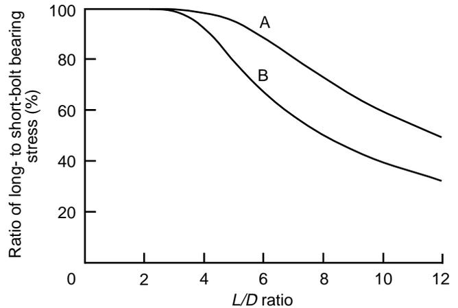
Figure 7-11. Variation in the proportional limit bolt-bearing stress parallel to grain with  $L/D$  ratio. Curve A, bolts with yield stress of 861.84 MPa (125,000 lb/in<sup>2</sup>); curve B, bolts with yield stress of 310.26 MPa (45,000 lb/in<sup>2</sup>).
