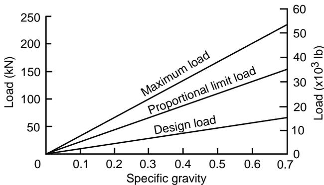
**Figure 7-18. Relation between load bearing parallel to grain and specific gravity (ovendry weight, volume at test) for two 101.6-mm (4-in.) split rings and a single 19.1-mm- (3/4-in.-) diameter bolt in air-dry material. Center member thickness was 127.0 mm (5 in.) and side member thickness was 63.5 mm (2-1/2 in.).**
